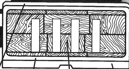
ABS Top Sheet    Fiberglass Torsion Box    Laminated Wood Core with Air Channels    Polyethylene Base
